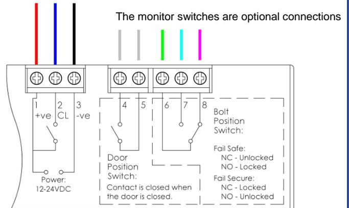
In either fail safe or fail secure configuration, maintained connection of '1' to '2' will keep the YD38 unlocked regardless of door position.
