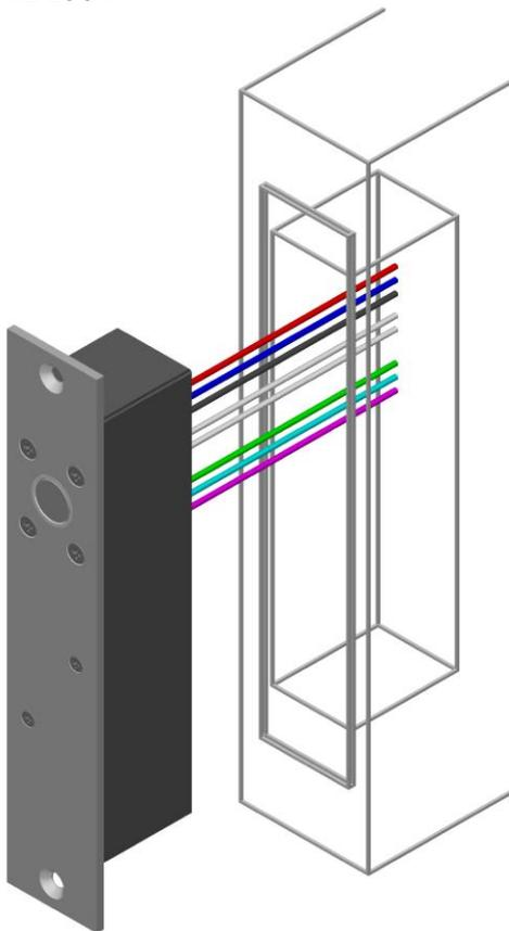
The wiring options and detail is shown overleaf. Once the desired wiring method is chosen run the wires into the rear of the mortice and connect to the lock. There are screw terminals for each wire and a connector guide is shown on the lock cover.
