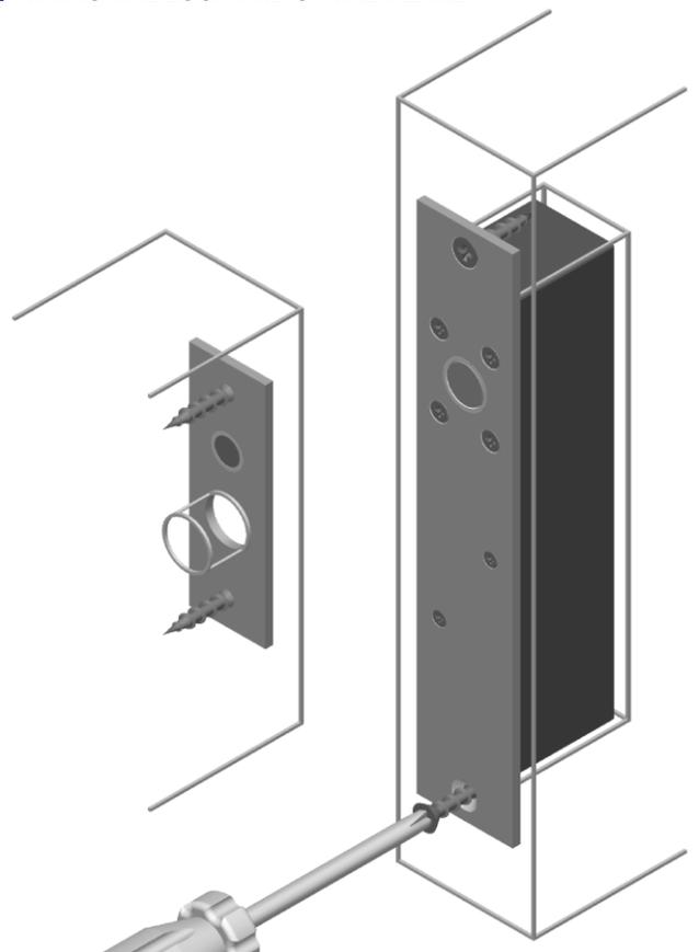
Slide the lock back into the mortice, making sure that the wiring integrity is maintained. Secure the lock and strike plate in place, using the supplied mounting screws. Ensure that the hole behind the strike plate is free from swarf and is deep enough to allow the lock pin to fully extend when locked.
