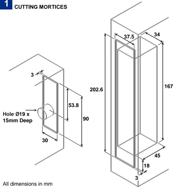
Cut mortices into the door and door frame for the strike plate and lock as per the dimensions shown. The top end of the strike plate must be aligned with the top of the lock so the bolt pin goes centrally into the hole in the strike plate. The gap between the lock face plate and strike plate must not exceed 6mm when the door is closed.
